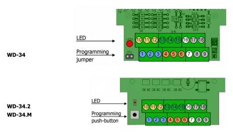
In order to set the address via the programming jumper / push-button perform the following steps:
