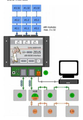
The interface (ZEUS) provides the connection between PC control. s88 modules and the BiDiB-nodes on the different levels of the system. The hub (BiDiB node 2) provides an additional level. BiDiB-nodes have different functions, e.g.: feedback modules (class "Occupancy") or stationary decoders (class "Accessory Control").
