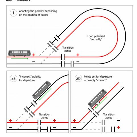
**Phase 1:** Train entering the terminal loop: When switching the points with the push-buttons or via the integrated points decoder, the polarity in the transmission zone and within the terminal loop is set automatically that way the train can enter the terminal loop without causing a short circuit. In case the position of points has not been altered since the last train has left, the polarity within the terminal loop is already set correctly.
