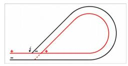
In digital layouts loop modules generally have to adapt the polarity within the terminal loop to the one outside. In case the polarity outside the terminal loop would be altered, different polarities would meet with each other at the transition to the next booster section. Thus the problem would be misaligned only.
