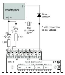
**Caution:** Never use LEDs without series resistors, as in this case the LEDs will be destroyed quickly.
