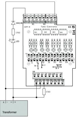
**Caution:** Never connect electric light bulbs to the outputs as these consume more than 50 mA current, as a rule. The outputs which are designed for a maximum current of 50 mA would be destroyed when putting them into operation.
