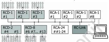
There are five different detectors connected to the data bus, all together controlling 13 separate track sections. In order to display and exploit the data there are used:
