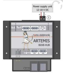
Use the supplied terminal block to connect the power supply. Connect the terminal to the "Power" connector so that the screws are visible from above.
