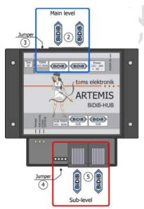
The two RJ 45 connection sockets on the main and sub levels are each connected in parallel. They can therefore optionally be used for connection to other BiDiB nodes of the respective level.
