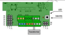
When connecting a node to the power supply the polarity is of no importance. In case several similarly designed decoders (e.g. WD-34. (M.)BiDiB, SD-34.BiDiB or MD-2.BiDiB) are connected to the same power supply, the assignment of ground / plus of the transformer or plus / minus of the power pack should be the same with all decoders.
