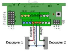
Connection of two decouplers to terminals 4 to 6
