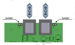
In case the Multi-Decoder MD-2.BiDiB is the last node in a level, you have to bypass the two 2-pole socket pins beside the RJ 45 connection sockets. The easiest way is to insert the jumpers included in the scope of supply.
