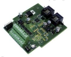
8- fold servo decoder and 4-fold turnout decoder
