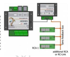
With this constellation (i.e. with one RCA-Bridge in a bus-line), you can connect 31 additional display devices RCA-1. In order to assign a RCA-1 to a track section, you have to program an address between 1 and 24 for the display device (see manual of the display device).
