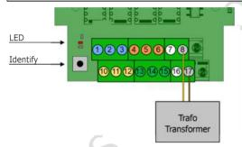
When connecting a node to the power supply the polarity is of no importance. In case several similarly designed decoders (e.g. WD-34.BiDiB and SD-34.BiDiB) are connected to the same power supply, the assignment of ground / plus of the transformer or plus / minus of the power pack should be the same with all decoders
