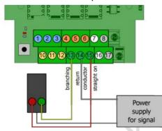
Connection of a signal to terminals 13 to 15 ("switching contacts 4")
