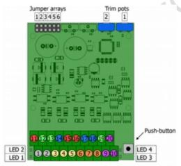
All settings are made via trim pots. The settings are saved in an IC on the circuit.
