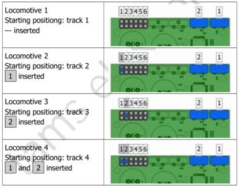
You can put locomotives 1 and 2 or locomotives 3 and 4 on the tracks at once, in order to program them one after the other. The tracks of the opposite terminus station always have to be open when changing into the programming mode.
