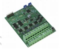
Shuttle-train control for analogue d.c. model railway layouts
