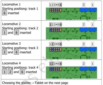
You can put locomotives 1 and 2 or locomotives 3 and 4 on the tracks at once, in order to program them one after the other. The tracks of the opposite terminus station always have to be open when changing into the programming mode.
