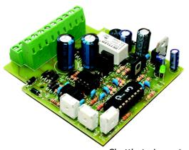
Shuttle-train control for analogue a.c. model railway layouts
