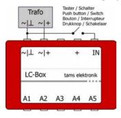
With some versions you can control the program flow or choose one of two different program variants via the switching input IN. According to the version and to the intended mode of operation you can use switches, push-buttons, fixed solder connections or upstream control modules (e.g. switching decoders). With some versions the switching input IN has no function.
