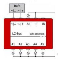
As a rule you can connect one or two bulbs to one output. Bulbs are not polarized. Connect one side to the output, the other to the return conductor (+).
