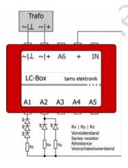
Examples for the connection of LEDs:
