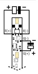
The minimum voltage sustaining capability of the goldcaps is 5,5 V. The minimum voltage sustaining capability of the capacitor depends on the power supply.
