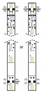
Solder the connecting wires for the power supply to the connecting points P1, P3, P5 or P7 (from the one rail / centre conductor) and the connecting points P2, P4, P6 or P8 (from the other rail / outer conductor). Follow the connection diagram.
