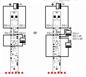
Choose an electrolytic capacitor or a goldcap with a capacity as high as possible. As the housings of electrolytic capacitors and goldcaps are bigger when the capacity is higher, the maximum capacity is limited by the space available to mount the capacitor.
